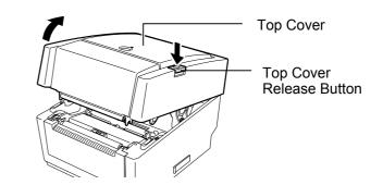
As the Top Cover is held by the damper, it does not close under its own weight.
